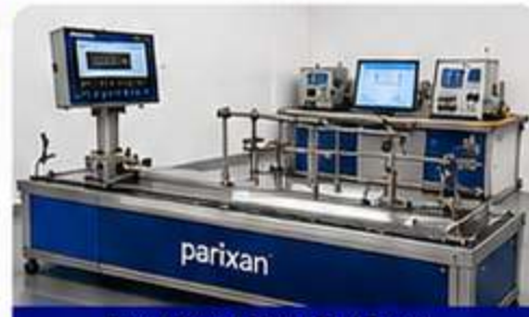
Flow / Water Meter Test Bench
